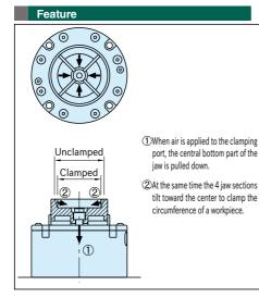
The diaphragm clamping mechanism allows securely clamping a workpiece with 4 jaw sections.
